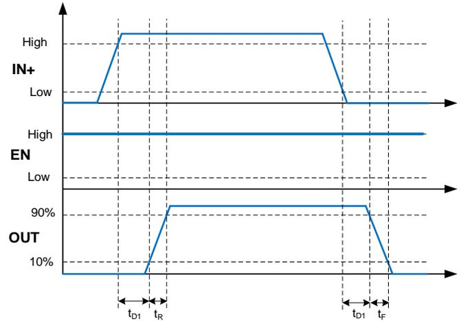
(PWM input to IN+ pin, EN pin tied to VDD)
